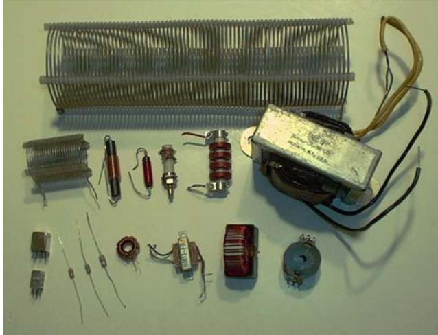
An assortment of inductors is shown on the left. The kinds usually used in modern homebrew ham equipment are in the bottom row. The tiny metal cans are shielded miniature IF transformers used in superhetrodyne receivers. The tiny chokes at the lower left resemble resistors and use the same color codes. I used lots of these in the designs in this book. The big coils, "chokes," and iron transformers were common in vacuum tube transmitters 50 years ago.
